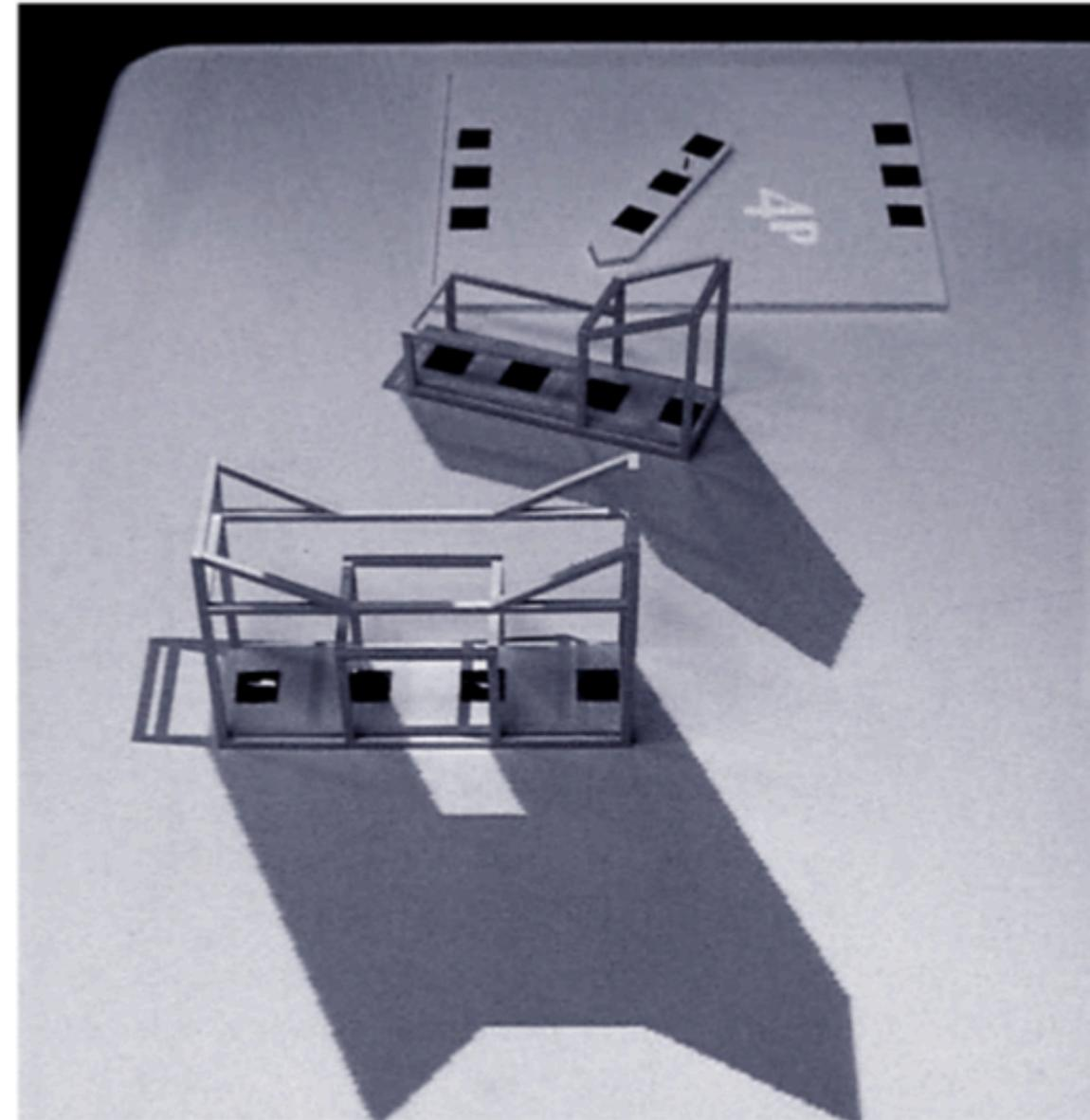
Urp and shadow simulation. Physical building models casting digital shadows, and a clock tool to control time of day (position of the sun).
