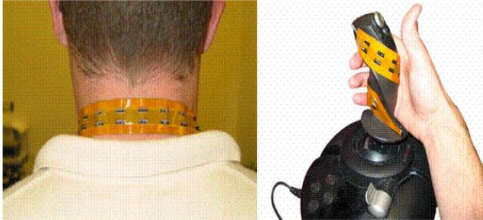
Tactile Display based on Shape Memory Alloy (MIT Touchlab)
