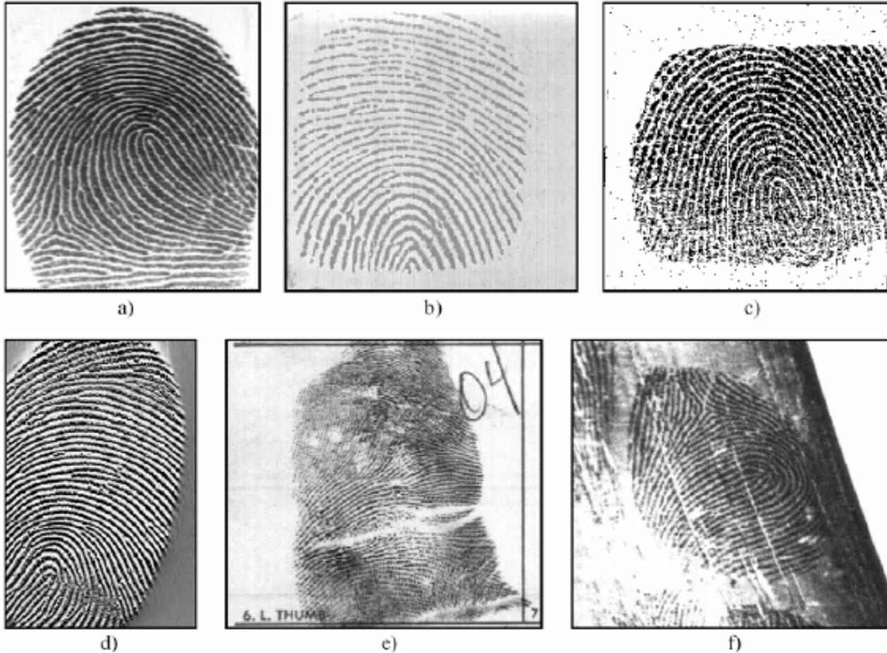
Fingerprint images produced by: a) optical scanner live-scan; b) capacitive scanner live-scan; c) piezoelectric scanner live-scan; d) thermal scanner live-scan; e) impression through ink off-line; f) latent fingerprint.
