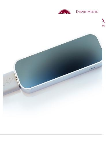
Leap motion - two monochromatic IR cameras and three infrared LEDs
