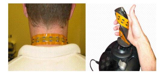
Tactile Display based on Shape Memory Alloy (MIT Touchlab)
