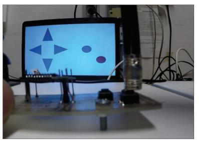
FIGURE 3. Button pressure on the battery-free mouse and corresponding action on the screen.
